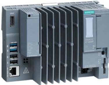
SIMATIC ET 200SP Open Controller, CPU 1515SP PC2 T, 8 GB RAM (basic device 6ES7677-2DB40-0AA0), 128 GB CFast with Windows 10 IoT Enterprise LTSC 2019 64-bit, and S7-1500 software Controller CPU 1505SP T V2x preinstalled; interfaces: 1x slot CFast, 1x slot SD/MMC, 1x connection for ET 200SP BusAdapter PROFINET, 1x 10/100/1000 Mbps Ethernet, 2x USB 3.0; 2x USB 2.0, 1x DisplayPort; documentation on CFast, restore image on CFast
