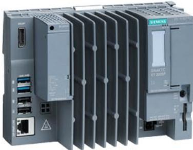
SIMATIC ET 200SP Open Controller, CPU 1515SP PC2, 8 GB RAM (basic device 6ES7677-2DB40-0AA0), 128 GB CFast with Windows 10 IoT Enterprise LTSC 2019 64-bit, and S7-1500 software Controller CPU 1505SP V2x preinstalled; interfaces: 1x slot CFast, 1x slot SD/MMC, 1x connection for ET 200SP BusAdapter PROFINET, 1x 10/100/1000 Mbps Ethernet, 2x USB 3.0; 2x USB 2.0, 1x DisplayPort; documentation on CFast, restore image on CFast
