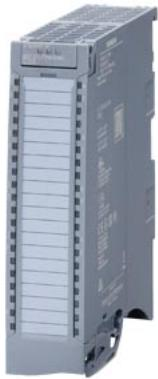
SIMATIC S7-1500, analog input module AI 8xHART HF, accuracy 0.1%, 8 channels in groups of 4, common mode voltage: 30 V AC/60 V DC, diagnostics; hardware interrupts calibrate in RUN; delivery including infeed element, shielding bracket and shield terminal
