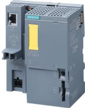
SIMATIC DP, CPU 1514SP F-2 PN for ET 200SP, central processing unit with 900 KB work memory for program and 3.5 MB for data, 1st interface: PROFINET IRT with 2-port switch, 2nd interface: PROFINET RT, 6 ns bit performance, SIMATIC Memory Card required, BusAdapter required for 1st interface
