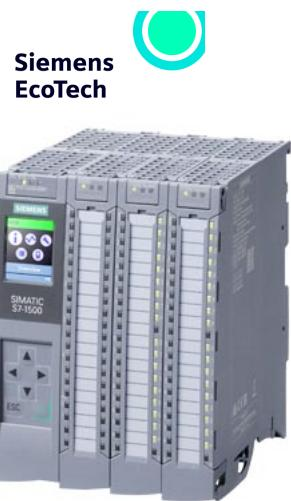
SIMATIC S7-1500 compact CPU, CPU 1512C-1 PN, central processing unit with work memory: 400 KB for program and 2 MB for data, 32 digital inputs, 32 digital outputs, 5 analog inputs, 2 analog outputs, 6 high-speed counters, 4 fast outputs for PTO/PWM/frequency output, 1st interface: PROFINET IRT with 2-port switch, 6 ns bit performance, including front connector push-in, SIMATIC Memory Card required
