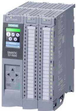
SIMATIC S7-1500 compact CPU CPU 1511C-1 PN, central processing unit with 300 KB work memory for program and 1.5 MB for data, 16 digital inputs, 16 digital outputs, 5 analog inputs, 2 analog outputs, 6 high-speed counters, 4 high-speed outputs for PTO/PWM/frequency output 1st interface: PROFINET IRT with 2-port switch, 6 ns bit performance, including front connector push-in, SIMATIC Memory Card required
