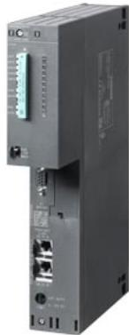
SIMATIC S7-400, CPU 416-3 PN/DP Central processing unit with: Work memory 16 MB, (8 MB code, 8 MB data), interfaces 1st interface MPI/DP 12 Mbit/s, (X1), 2nd interface Ethernet/PROFINET (X5) 3rd interface IF 964-DP plug-in (IF1)
