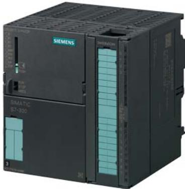
\*\*\*spare part\*\*\* SIMATIC S7-300, CPU 317T-3 PN/DP, central processing unit for PLC and technology tasks, 1024 KB work memory, 1st interface MPI/DP 12 Mbps, 2nd interface DP (drive), 3rd interface Ethernet PROFINET with 2-port switch, integrated I/O for technology, front connector (1x 40-pole) and Micro Memory Card min. 8 MB required
