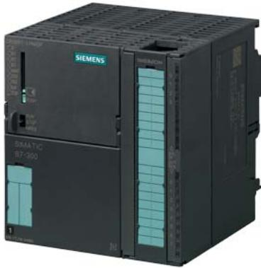
\*\*\*spare part\*\*\* SIMATIC S7-300, CPU 315T-3 PN/DP, central processing unit for PLC and technology tasks, 384 KB work memory, 1st interface MPI/DP 12 Mbps, 2nd interface DP (drive), 3rd interface Ethernet PROFINET with 2-port switch, integrated I/O for technology, front connector (1x 40-pole) and Micro Memory Card min. 8 MB required
