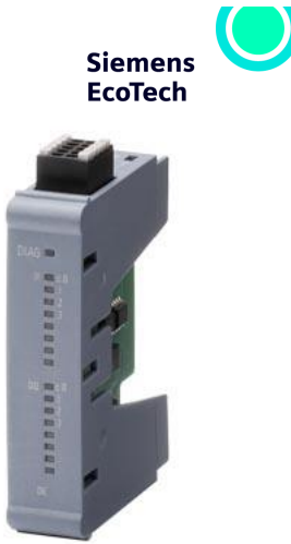
SIMATIC S7-1200 G2: SB 1232 analog output, 4 AO, outputs: 4 x AQ 14 bit DAC (+/-10 V, 0-20 mA or 4-20 mA)
