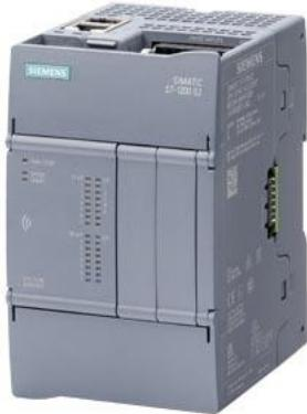
SIMATIC S7-1200 G2: compact CPU 1214C DC/DC/RLY; power supply: DC 20.4-28.8 V DC; onboard I/O: 14x DI 24 V DC; 10 DO relay 2 A; memory: program 250 KB data: 750 KB, retentivity: 20 KB
