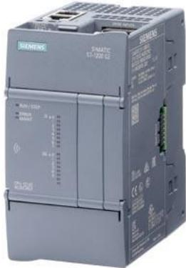
SIMATIC S7-1200 G2: compact CPU 1212C DC/DC/DC; power supply: DC 20.4-28.8 V DC; onboard I/O: 8x DI 24 V DC; 6x DO 24 V DC; memory: program 150 KB data: 500 KB, retentivity: 20 KB
