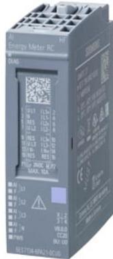
SIMATIC ET 200SP, analog input module, AI Energy Meter RC HF, for Rogowski coils or current/voltage transformer 333 mV, with network analysis functions, suitable for BU type U0, channel diagnostics
