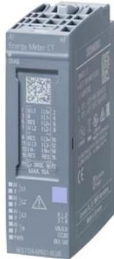
SIMATIC ET 200SP, analog input module, AI Energy Meter CT HF, for 1A or 5A current transformer, with network analysis functions, suitable for BU type U0, channel diagnostics
