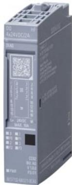
SIMATIC ET 200SP, digital output module, DQ 4x24 V DC/2 A high feature, source output (PNP, sourcing output) packing unit: 1 unit, suitable for BU type A0, color code CC02, channel diagnostics for: short-circuit and wire break, supply voltage, channel fault LED
