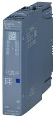
SIMATIC ET 200SP HA, analog output module, AQ 4XI HART isol suitable for terminal block K0, L0, color code CC00, channel diagnostics, 16-bit, +/-0.1%
