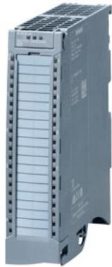
SIPLUS S7-1500 AI 8xU/I HF based on 6ES7531-7NF00-0AB0 with conformal coating, -40...+70 °C, start up -25 °C, analog input module 16-bit resolution, accuracy 0.1%, 8 channels in groups of 1, common mode voltage: 30 V AC/60 V DC, diagnostics; hardware interrupts; including infeed element, shielding bracket and shield terminal
