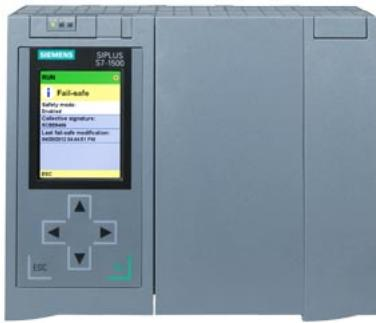
SIPLUS S7-1500 CPU 1518F-4 PN/DP based on 6ES7518-4FP00-0AB0 with conformal coating, 0...+60 °C, central processing unit with work memory 4.5 MB for program and 10 MB for data, 1st interface: PROFINET IRT with 2-port switch, 2nd interface, Ethernet, 3rd interface, Ethernet, 4th interface, PROFIBUS, 1 ns bit performance, SIMATIC Memory Card required
