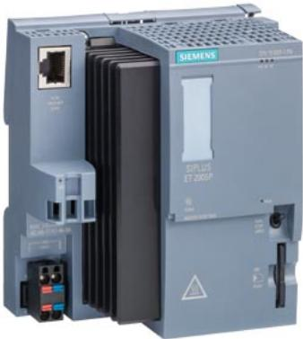
SIPLUS ET 200SP CPU 1510SP-1 PN based on 6ES7510-1DJ01-0AB0 with conformal coating, -40...+70 °C, no pluggable BusAdapter, central processing unit with work memory 100 KB for program and 750 KB for data, 1st interface, PROFINET IRT with 3-port switch, 72 ns bit performance, SIMATIC Memory Card required,
