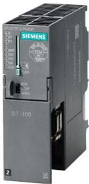
\*\*\*spare part\*\*\* SIPLUS S7-300 CPU 317F-2PN/DP based on 6ES7317-2FK14-0AB0 with conformal coating, -25...+60 °C, central processing unit with 1.5 MB work memory, 1st interface MPI/DP 12 Mbps, 2nd interface Ethernet PROFINET, with 2-port switch, Micro Memory Card required
