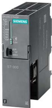
\*\*\*spare part\*\*\* SIPLUS S7-300 CPU 315F-2PN/DP based on 6ES7315-2FJ14-0AB0 with conformal coating, -25...+60 °C, central processing unit with 512 KB work memory, 1st interface MPI/DP 12 Mbps, 2nd interface Ethernet PROFINET, with 2-port switch, Micro Memory Card required
