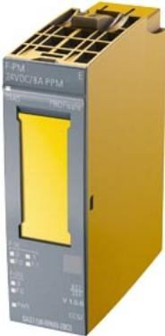
SIPLUS ET 200SP F-PM-E 24VDC/8A PPM based on 6ES7136-6PA00-0BC0 with conformal coating, -30...+60 °C, fail-safe power module PROFIsafe, 24 V DC safe shutdown of DQ and F-DQ up to PL D/SIL2 or PL E/SIL3 2 safe digital inputs 1 safe digital output PPM
