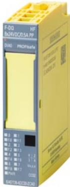
SIPLUS ET 200SP F-DQ 8x24VDC/0.5A PP HF based on 6ES7136-6DC00-0CA0 with conformal coating, -30...+60 °C, fail-safe digital outputs Cat. 4, PL e (EN ISO 13849-1) up to SIL 3 (IEC 61508)
