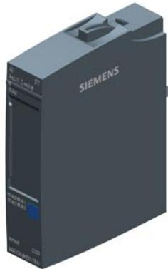
SIPLUS ET 200SP AI 4xU/I 2-wire ST based on 6ES7134-6HD01-0BA1 with conformal coating, -40...+70 °C, analog input module, suitable for BU type A0, A1, color code CC03, module diagnostics, 16 bit, +/-0.3%
