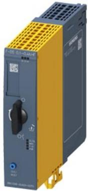
Fail-safe direct-on-line starter High Feature; Electronic switching; Electronic overload protection up to 0.09 kW / 400 V; Adjustment range 0.1 .. 0.4 A; PROFInergy; Option: 3DI/LC module
