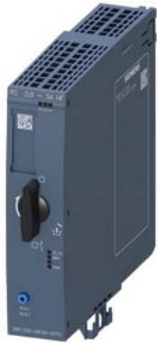
Reversing starter High Feature; Electronic switching; Electronic overload protection up to 1.1 kW / 400 V; Adjustment range 0.9 .. 3 A; PROFenergy; Option: 3DI/LC module
