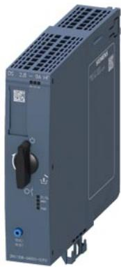
Direct-on-line starter High Feature; Electronic switching; Electronic overload protection up to 4 kW / 400 V; Adjustment range 2.8 .. 9 A; PROFenergy; Option: 3DI/LC module
