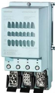
ET 200pro EDSE/DSSE HF electronic direct-on-line starter electronic (soft-) switching full motor protection consisting of: electronic overload protection + thermistor 400 V 3 AC/0.9 kW 0.15 A...2.00 A without brake contact 4 DI Han Q4/2 - Han Q8/0
