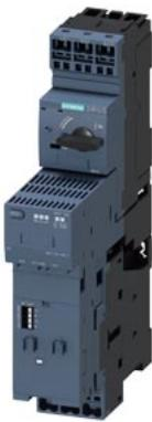
intelligent load feeder direct starter high feature 3.5-32 A up to 690 V AC type of coordination 2 frame size S0 for ET 200SP system consisting of 3RC7140-4EE11, 3RV2321-4EC20, 3RT2027-2BB40
